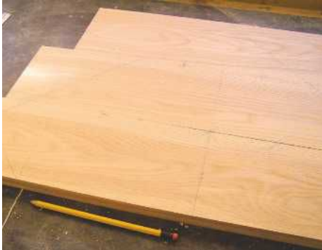
▲ Pic.1 Having planed the boards to size, mark out the top and bottom panels to determine the positions of the biscuits
